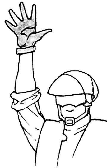
Go. "Execute orders." An upraised hand with fingers spread, palm forward. Final signal issued.
